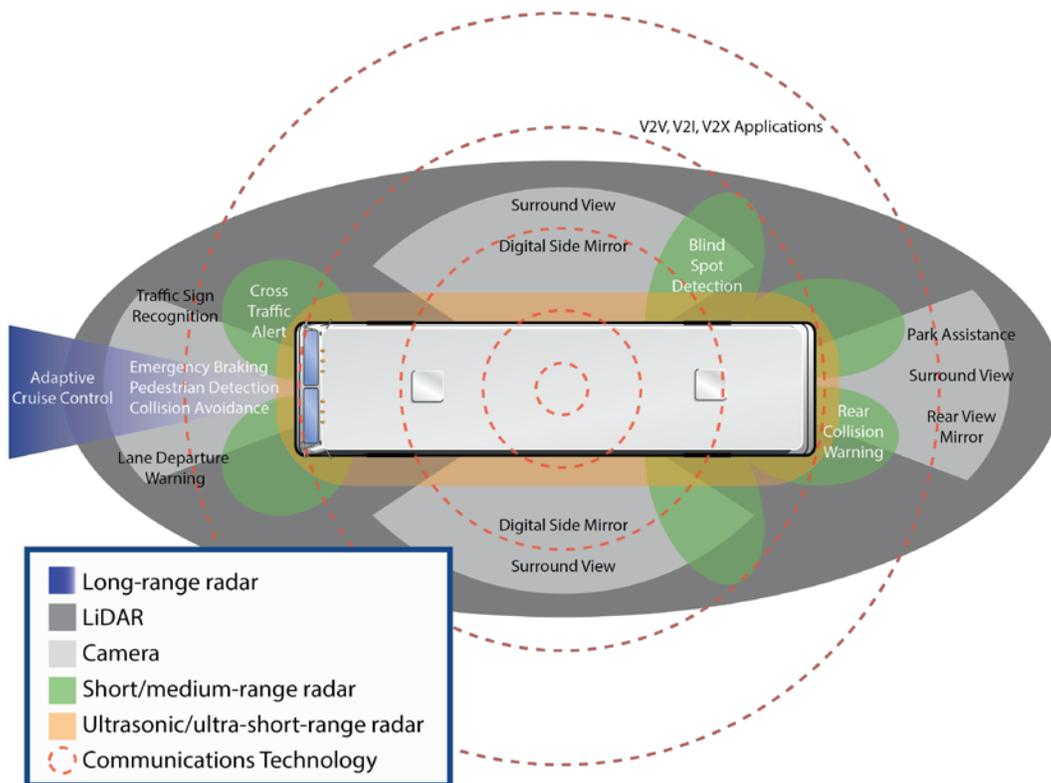
**Figure 1. Vehicle Automation Technologies (image Adapted from the Texas Instruments ADAS Solutions Guide)<sup>9</sup>**
