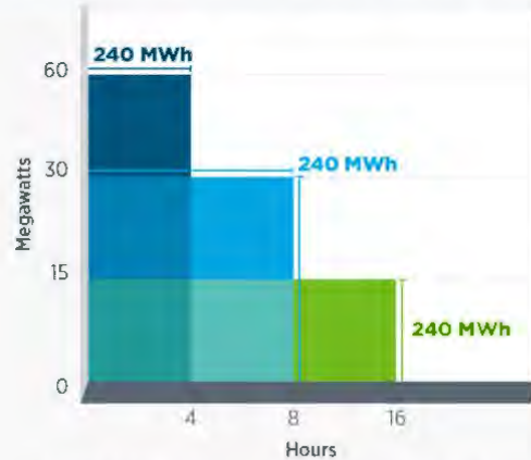
Figure 7: Energy storage use can depend on time and power output requirements. Source: Department of Energy
