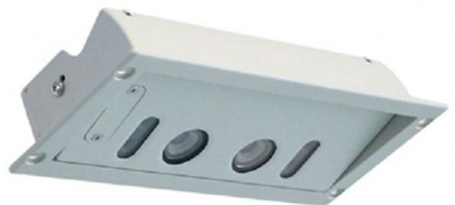
APC Technology Using Digital Cameras (Source: https://www.pcb.its.dot.gov/factsheets/apc/apc_overview.aspx#page=tech )
